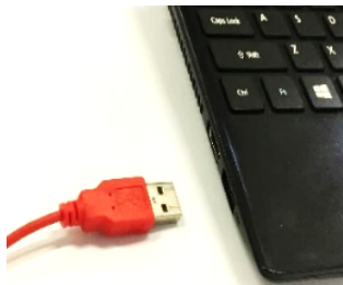
Figure 3: A standard USB A plug. This connects the Makey Makey to a computer.
